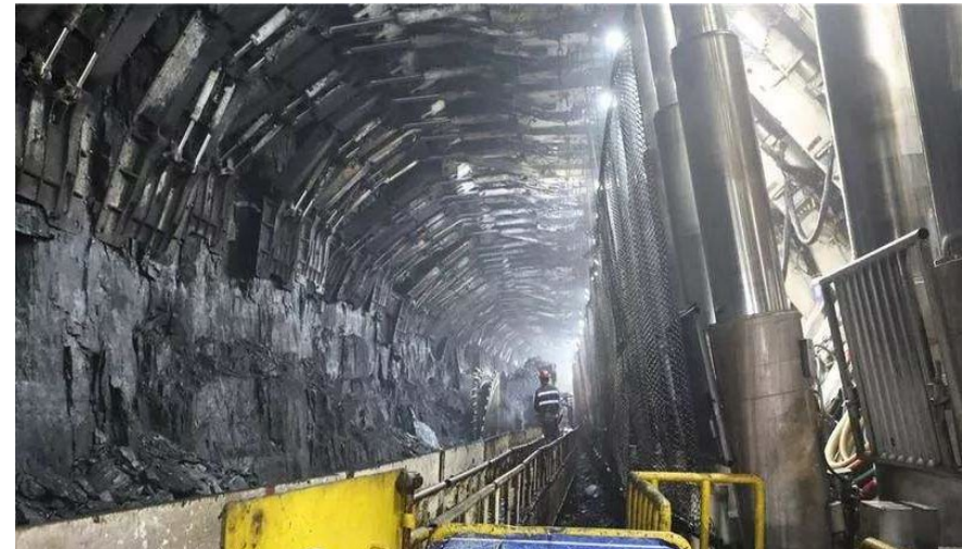
World's first 8.8 meter ultra-high mining face (Shangwan Coal Mine, China)
