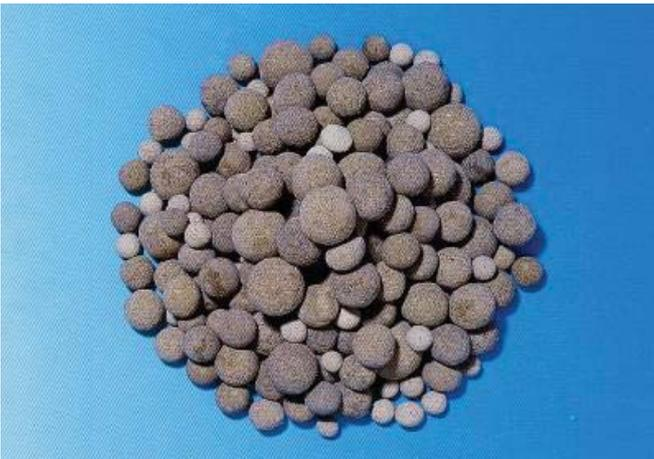
Photo 2 Artificial aggregate fabricated from coal ash (Toughlite)
