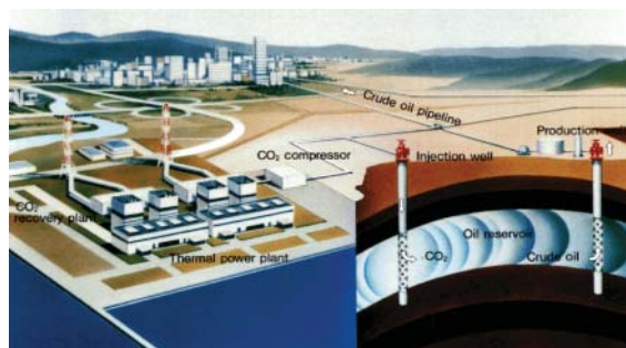
Photo 1 Conceptual view: CO 2 recovery from power plant flue gas for EOR
