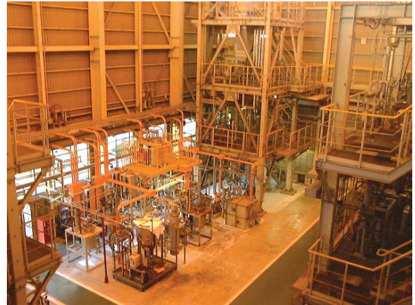
Photo 3 Test apparatus for continuous manufacturing of Hyper-coal
