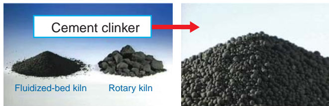
Photo 1 Clinker produced from a fluidized-bed kiln
