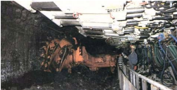
Longwall mining (SD Mining) drum shearer and shield support
