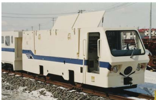
High-speed manned cars (former Taiheiyo coal mine)
