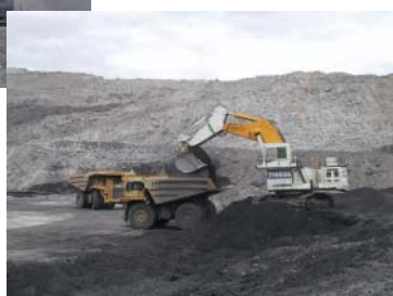
Power shovels & dump trucks
