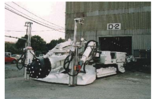
Drifting road header MRH-S220
