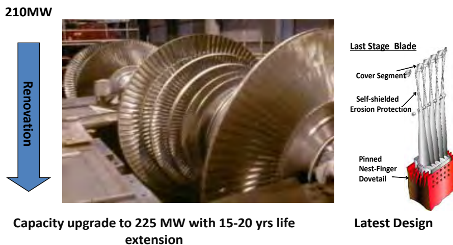
Figure 67. Turbine Restoration (Case 2) 47
