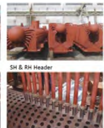
Bank Tube Rehabilitation
