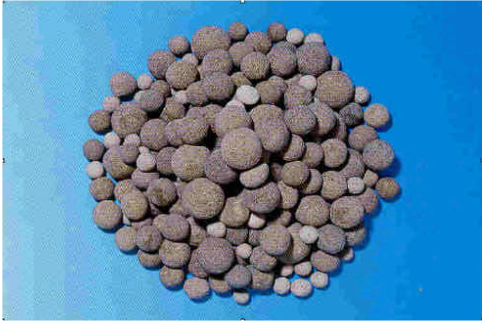
Figure 2. Manufactured Artificial Aggregate based on Coal Ash
